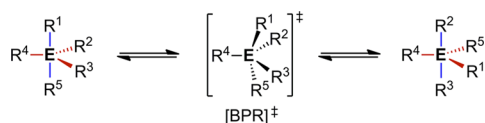
Figure 1. BPR as fundamental process for configurational changes in trigonal-bipyramidal compounds. 5 Axial substituents: blue; equatorial substituents: red.
